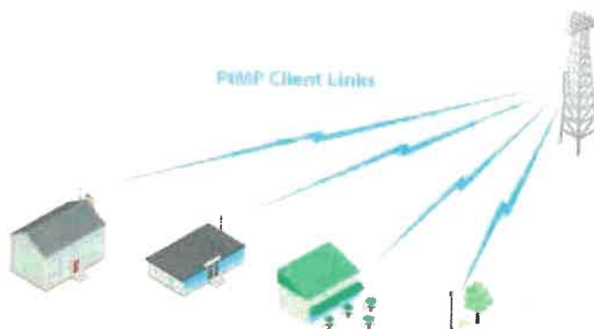
NanoStationM as powerful clients in an airMAX PtMP (Point-to-Multi-Point) network setup.
